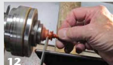
12 Hold the finial as you part it off the lathe. Note the small tenon at the base of the finial, which provides a good fit into the opening of the ornament body.
