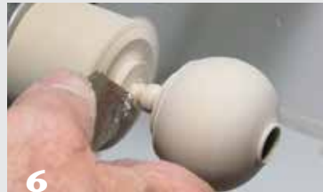
6 Part the globe from the waste block. Turn the lathe speed down and, as the globe just starts to wobble, cup it with your right hand and catch it as it comes free. Alternatively, part it most of the way through, turn off the lathe, and finish parting with a fine-tooth handsaw.
