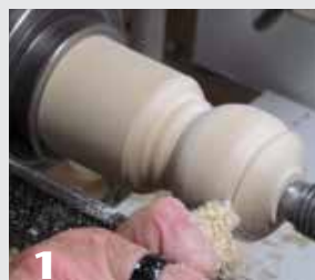
1 With the wood mounted in a chuck, shape the outside of the ornament globe. I use a \frac{3}{8} " (10mm) spindle gouge.
