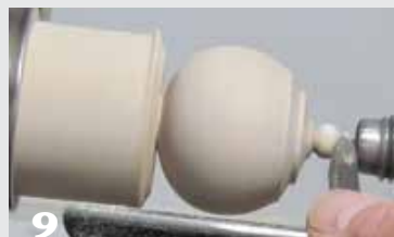
9 The tailstock live center brought gently in contact with the top will hold the globe in place as you finish the top. The small divot left by the center point can be dressed with a bit of abrasive and will leave a handy reference point to drill the hole for a screw eye.
