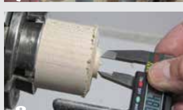
8 A snug fit makes a good jam chuck to finish turning the top of the ornament globe.
