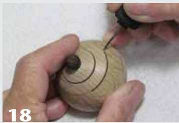
17 Rather than trying to “draw” lines with the burner as you would with a pencil, touch the tip of the stylus to the line and pull it away quickly at a ninety-degree angle. This will result in a more organic-looking line. With the low temperatures used here, burn flash should not be a problem. If you get discoloration, it is easily and cleanly removed by scraping with a small blade. Avoid sanding if at all possible.
