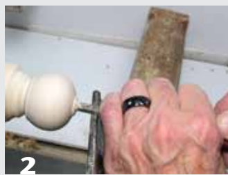
2 Leave a good mass of wood between the globe and chuck for added stability during hollowing.
