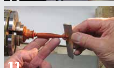
11 Finish the bottom of the drop finial using a detail gouge and, after the tailstock is removed, a bit of abrasive to remove the small divot from the tailstock live center.
