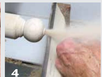
4 A blast of air will remove the shavings from inside.
